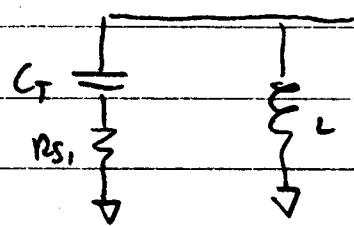
$$C_T = \frac{C_1 C_2}{C_1 + C_2} \quad (\text{series caps})$$
