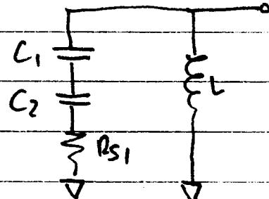
$$R_{S1} = \frac{X_1^2}{R_{pi}} = \frac{1}{R_{pi}} \left( \frac{1}{\omega C_2} \right)^2$$
