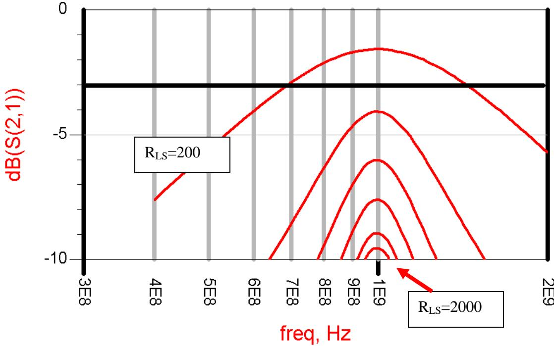
$$S_{21} (\text{dB}) = 20 \log(2V_{out}/V_{in})$$
