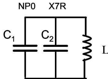
The equation below shows how the TCs of individual components combine<sup>1</sup>. Suppose that the inductor was resonated with a drift free capacitor (NP0). The frequency drift will be – 25 ppm/C. If the design frequency is 100 MHz, this corresponds to a drift of 2.5 kHz/C. But, the equation shows that you can set the total frequency TC (TCF) of a circuit to zero by combining capacitors with different TCs.
