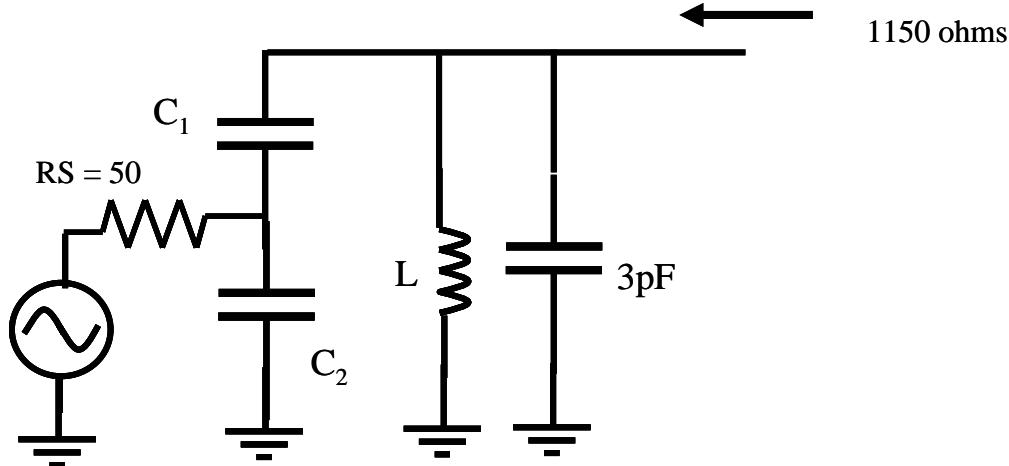
Because L is known, we can calculate the required  $C_{total}$  to resonate at 159 MHz.
