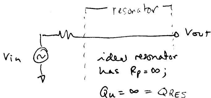
If  $R_p$ , the parallel equivalent of component loss is finite, then  $V_{out} < V_{in}$ .
