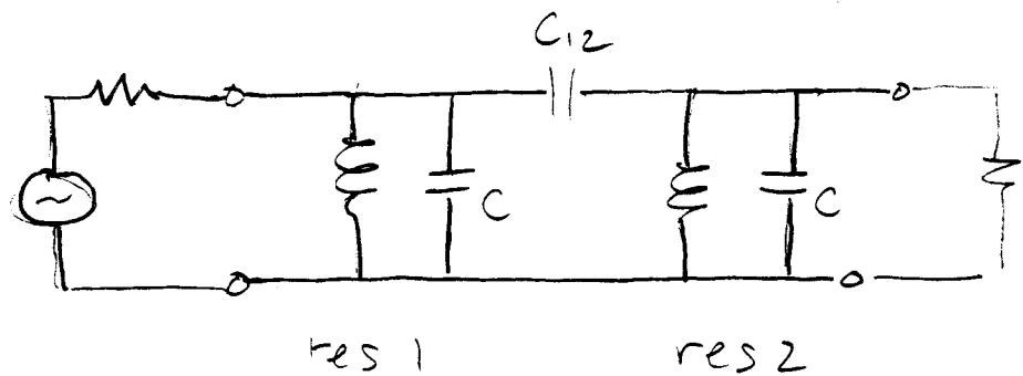
$$C_{12} = \frac{C}{Q} \quad Q = Q_L \text{ of single resonator}$$
