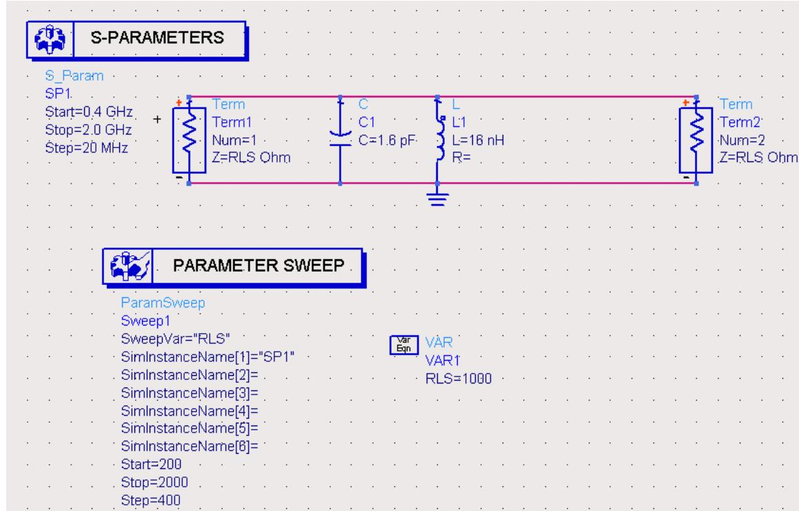
Loaded Q varies from 1 to 10 with the given parameter sweep.
