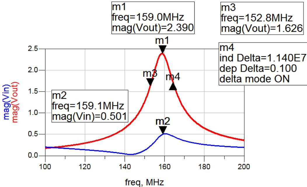
Everything looks as expected except for the bandwidth, 11.4 MHz rather than 10 MHz. This is due to the effect of  $R_P$ . If it mattered, we could go back through again and include this effect and get a 10 MHz BW, but most applications as this one are not so critical. The important thing is to get the correct impedance transformation.
