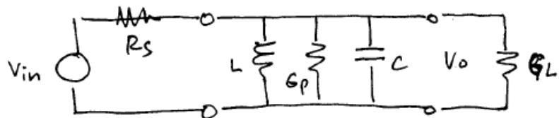
$$\text{total } Q = \frac{\omega_0 C}{G_S + G_P + G_L} = Q_L \text{ or } \underline{\text{loaded } Q}.$$
