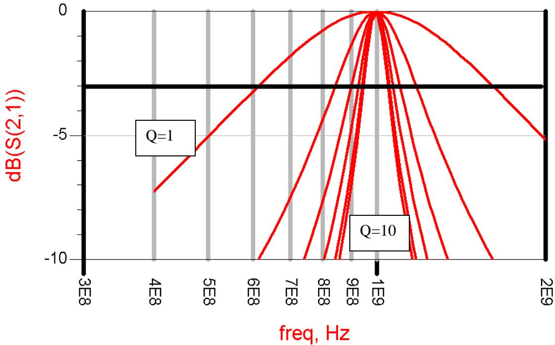
Now, the circuit is modified to include a 500 ohm resistor ( $R_P$ ) in parallel with the LC network. This resistance represents the parallel equivalent loss due to both the L and the C. So, now we have a finite unloaded Q.
