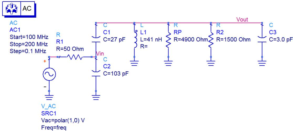
A small signal AC simulation is performed which includes the RP and excess C of the load. If the load is matched correctly to the source, we should see half of the source voltage at node Vin, 0.5V (available power). Vout should be  $4.8 \times 0.5 = 2.4V$ .
