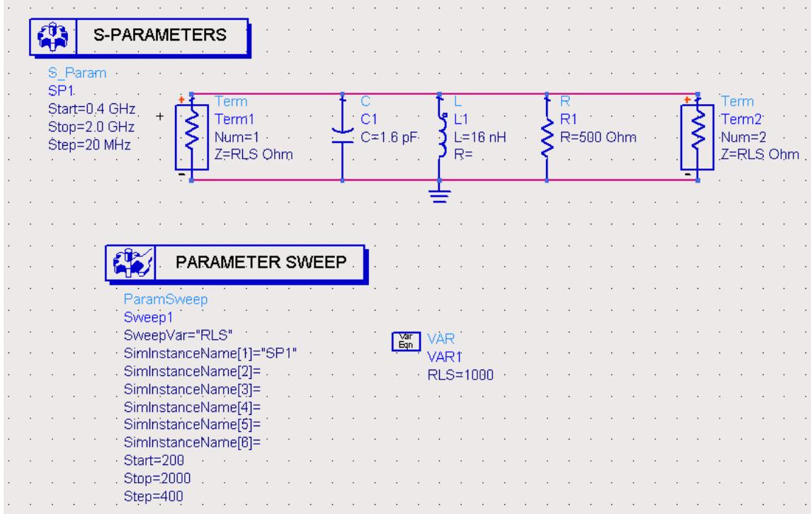
Note that the insertion loss increases as loaded Q,  $Q_L$ , approaches  $Q_U$ . Sweeping RLS, we see at resonance, the reactances cancel, and we are left with a resistive divider.
