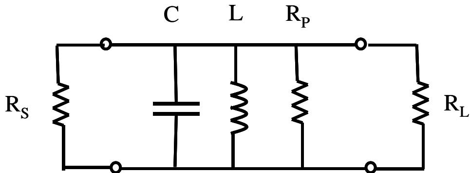
Here is a parallel resonant circuit ( $C, L$  and  $R_P$ ) connected to the outside. The total  $Q$  of this circuit is called the loaded  $Q$  or  $Q_L$  and is given by
