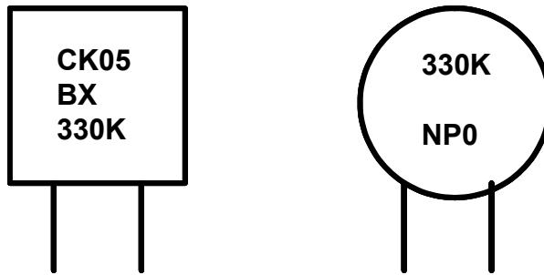
The two leaded capacitors above illustrate the labels found on typical capacitors of the X7R and NP0 types. The value is given by the numerals: 330. In this example, this is 33 pF. It goes 1<sup>st</sup> significant digit (3), 2<sup>nd</sup> significant digit (3), and multiplier ( $10^0$ ). The letter K is the tolerance, which is +/- 10%.
