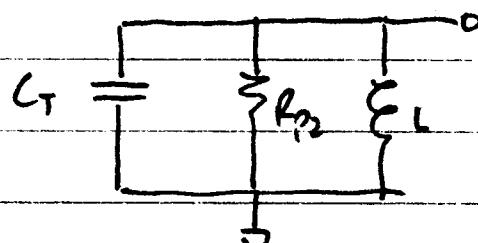
$$R_{S2} = \frac{X_2^2}{R_{pi}} = \frac{1}{R_{pi}} \left( \frac{1}{\omega C_T} \right)^2$$
