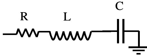
At resonance, the reactances cancel out leaving just a peak voltage,  $V_{pk}$ , across the loss resistance, R. Thus,  $I_{pk} = V_{pk}/R$  is the maximum current which passes through all elements. Then,
