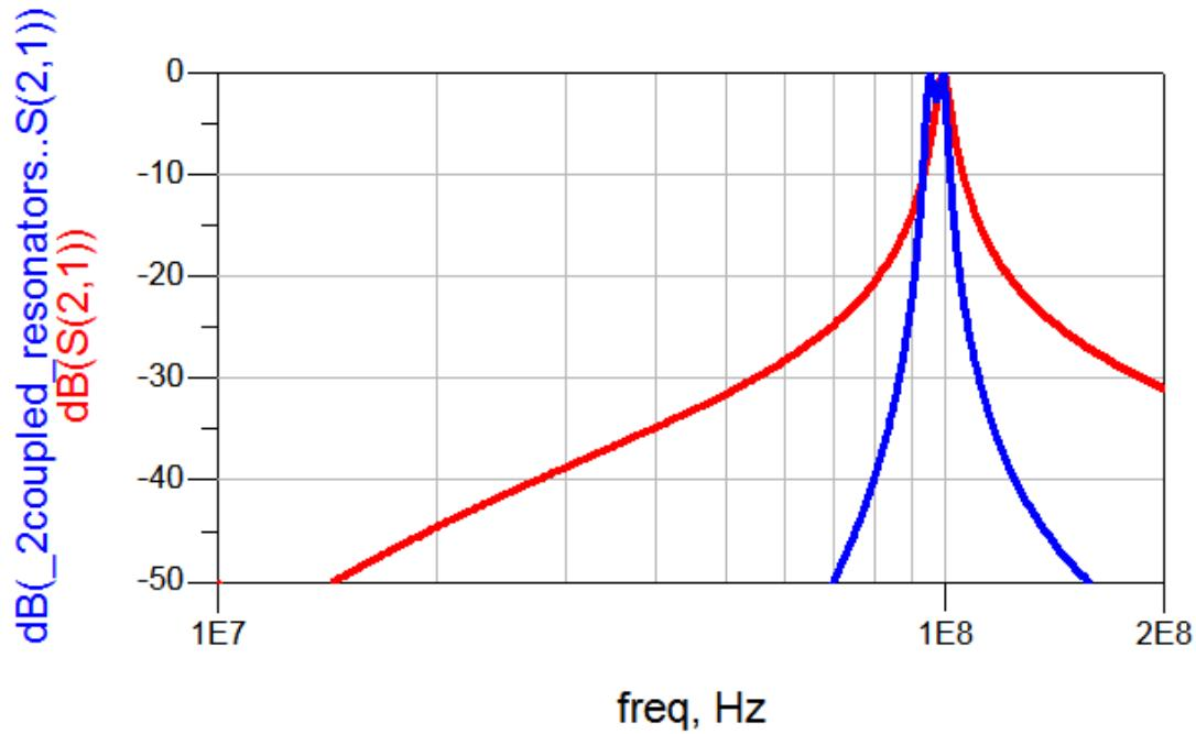
Note the improvement in the stopband rejection provided by the coupled resonator compared with the single resonant tapped C circuit.
