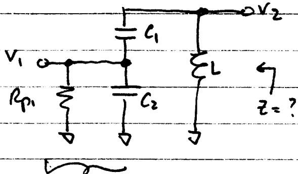
This network can be used as an impedance transformer.
